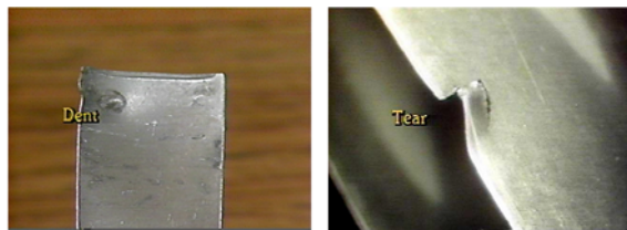
Figure 2-16. Compressor FOD Damage
