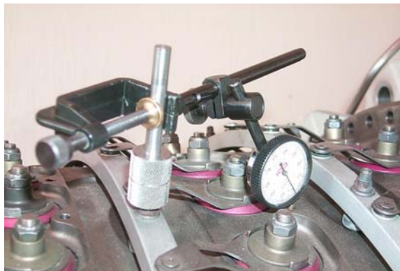
Figure 2-47. Typical Dial Indicator Set up
