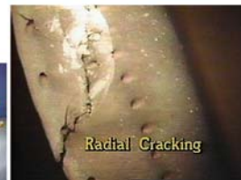
Figure 2-33. Typical Radial Cracking
