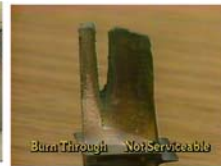
Figure 2-32. Typical Burn Through
