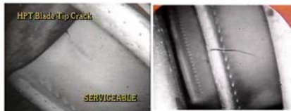
Figure 2-34. HPT Blade Crack Serviceable
